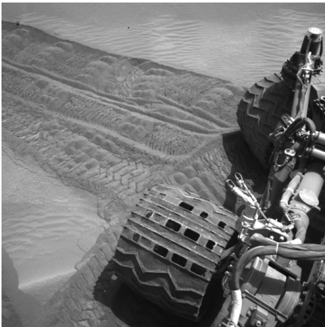
Figure 24. Sol 711 NavCam image of the RM and RR wheel after a turn-in-place command timed out. According to IMU data, the turn slip was 40.4%.
