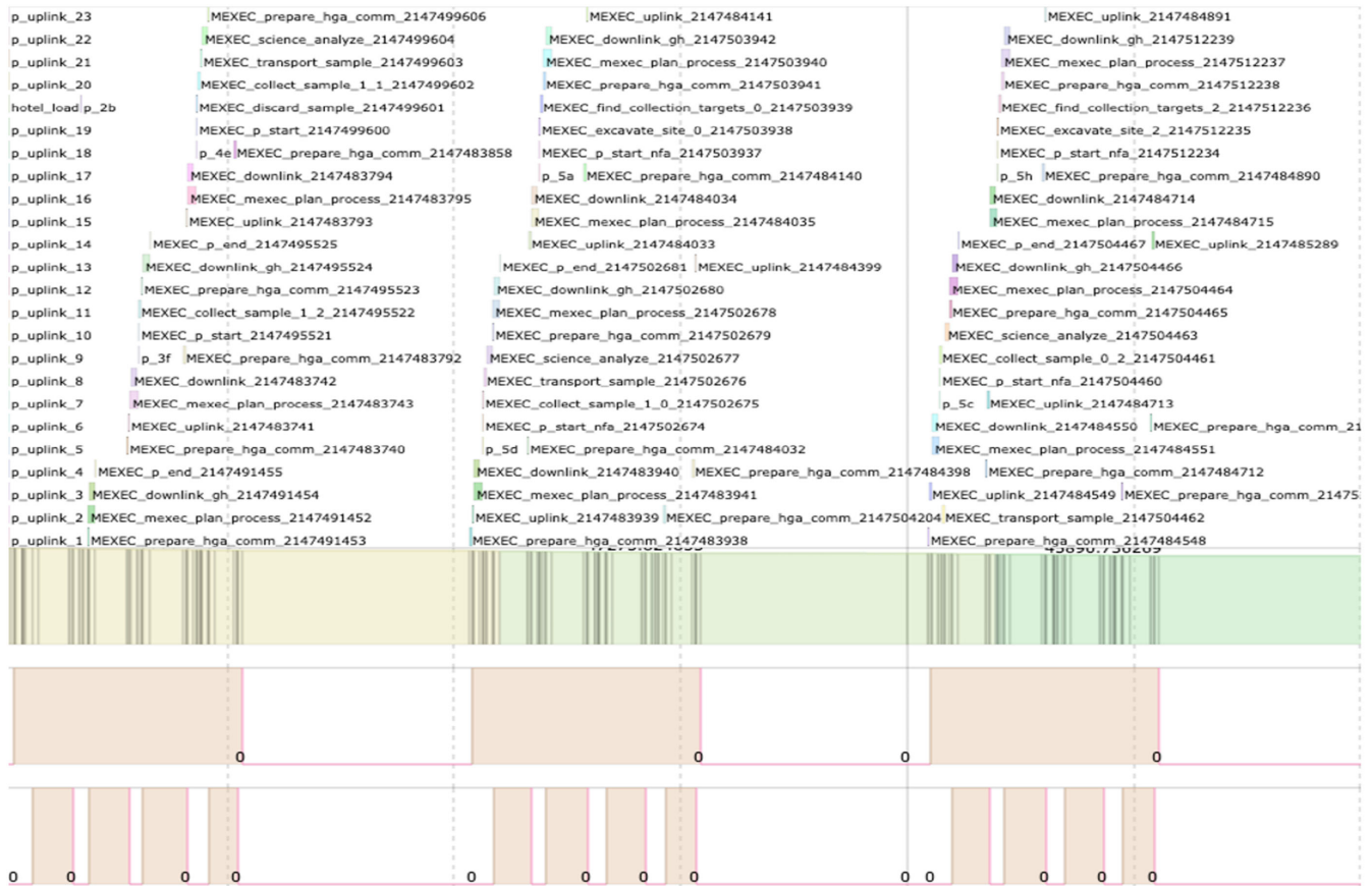
Fig. 8 Sample of a full mission schedule: 3 sites excavated, 9 samples collected over multiple sols, plus episodic imagery, fixed exogenous uplink windows, and downlinks. Mission ends when battery depleted.
