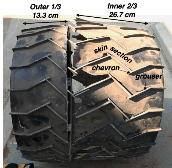
Figure 16. MSL Flight Wheel with 19 Broken Grousers.
