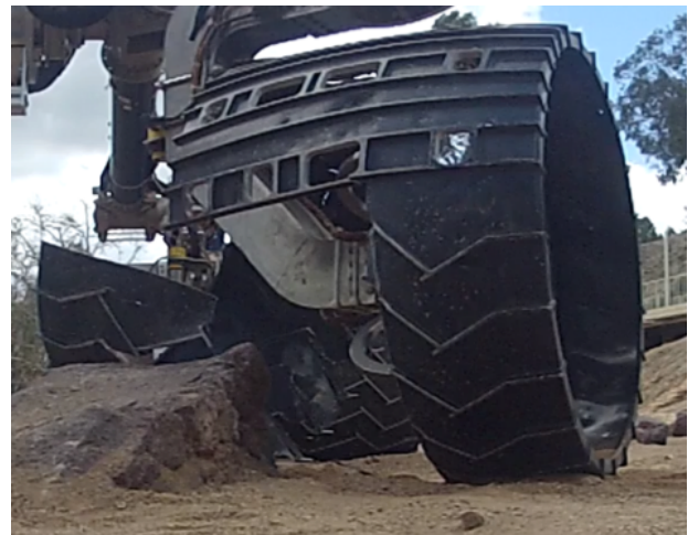
Figure 22. Unconstrained LF portion pinned to the rock.
