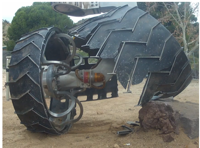
Figure 21. Rotated LF After Break 1.
