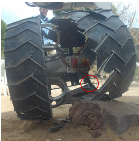
Figure 20. Rotated LF Prior to Break 1. Break Location 1 Circled.
