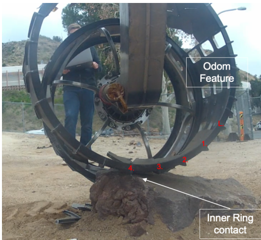
Figure 19. LF after being driven onto the shed rock.
