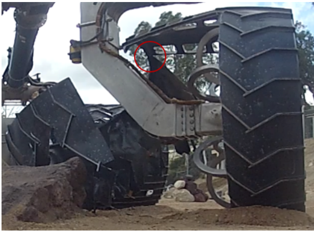
Figure 23. Unconstrained LF During the Pigeon-Toe Maneuver. Break Location 2 Circled.
