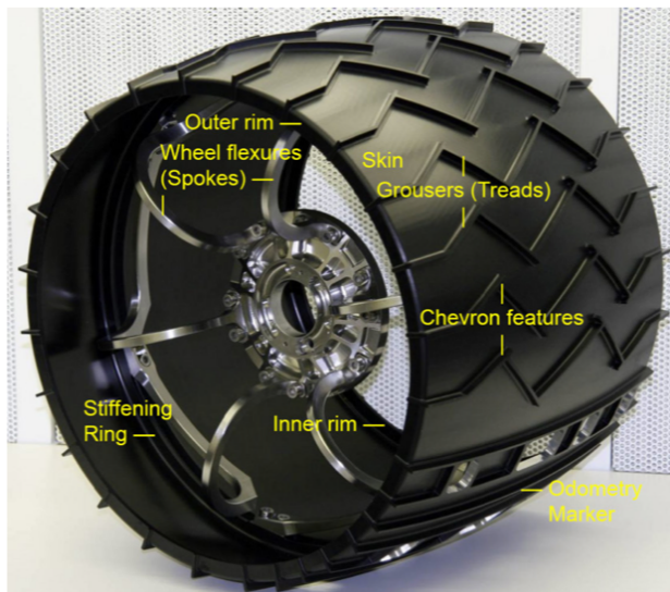
Figure 2. Features of an MSL Flight Wheel.
