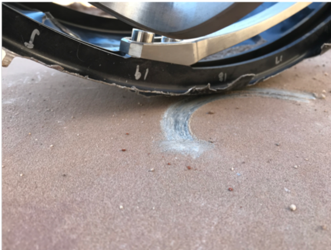
Figure 15. Contact Point of a Rimmed Wheel Due to Steer Axis Offset.
