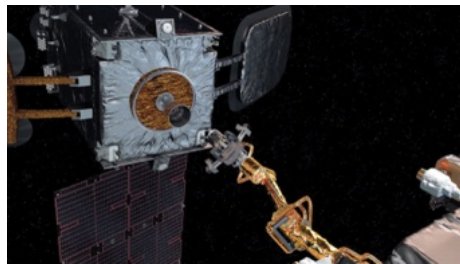
Figure 2: NASA’s conceptual servicing spacecraft, extends its robotic arm to grab and refuel a satellite. [4]
