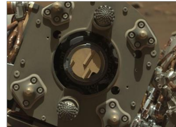
Mars 2020's abrasion drill bit. NASA/JPL-Caltech/ASU
