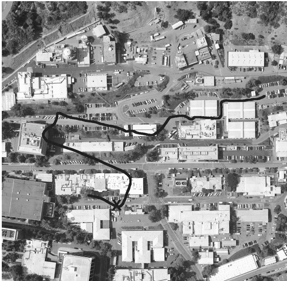
Figure 2: The result of Visual Odometry overlaid on the overhead imagery. X marks the actual traverse end point.
