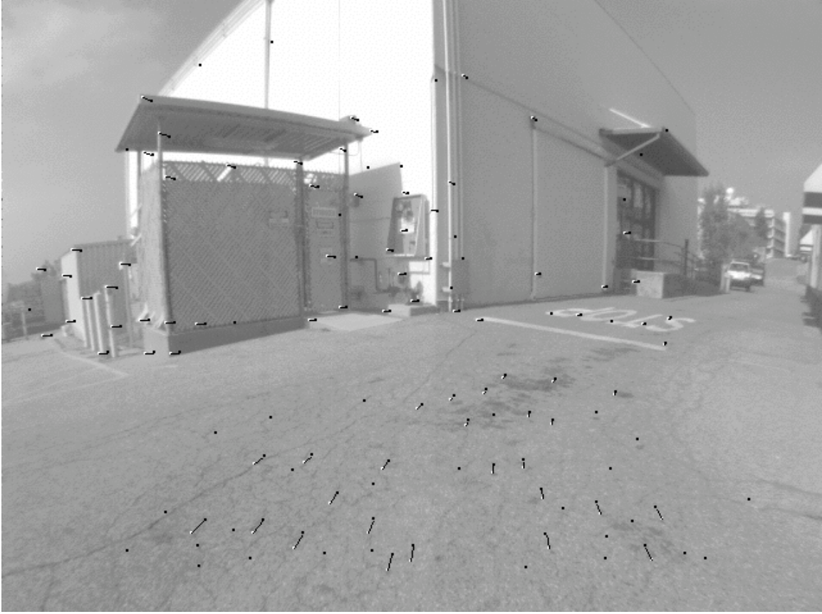
Figure 1: Example of features used by Visual Odometry. The vectors show the displacement of features between sequential images. In this image, one can see there is both forward camera motion (as evidenced by those features on the ground) as well as a strong rotational component (as evidenced by those features lying on the buildings).
