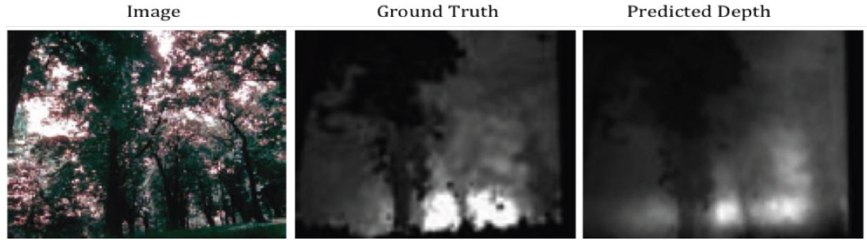
Figure 2.4: Example results from our deep network based depth regression scheme. (Left) Image, (Middle) Ground truth (Right) Predicted depth map.
