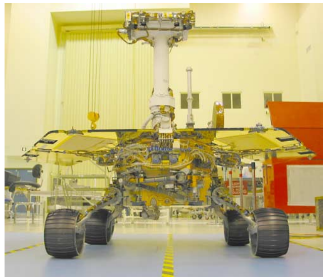
Figure 9. The MER 2 rover, during integration at testing at the Jet Propulsion Laboratory in Pasadena, California. The Navcams (pointing down in this picture) are at the top of the Pancam Mast Assembly. The Front Hazcams are at the center of the picture. Scale: The wheels are 25 cm high and the Navcams are ~1.5 m above the floor.
