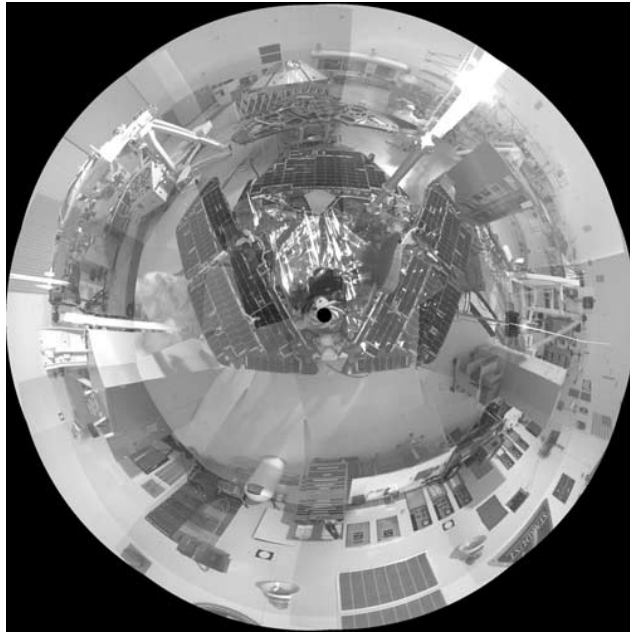
Figure 28. Navcam polar projection mosaic, looking down onto the MER 2 flight rover, acquired during an imaging test in the Payload Hazardous Servicing Facility at Kennedy Space Center in Florida. Despite the poor lighting conditions experienced during the acquisition of this panorama (and the movement of test personnel during the panorama), the resulting composite image is a good example of the automated mosaic production capability of the JPL MIPL ground software. This image is composed of 10 individual Navcam images. Note that there has been no radiometric correction done to the individual images.
