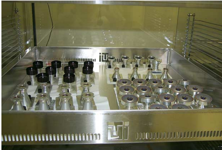
Figure 1. Mars Exploration Rover (MER) camera optics, during the camera assembly process. The Navcam lens assemblies are at the upper left, the Pancam lens assemblies at the lower left, the Hazcam lens assemblies at the middle right, and the Descent camera lens assemblies are at the top right corner.
