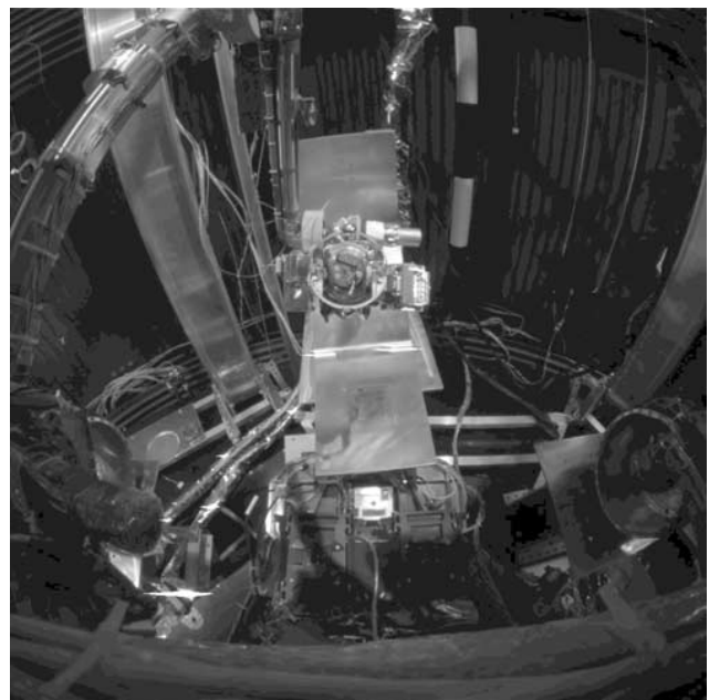
Figure 20. The Instrument Deployment Device (IDD) workspace, as viewed from the front left Hazcam camera during MER 1 System Thermal Test. Note the IDD turret with the Rock Abrasion Tool (RAT) toward the camera.
