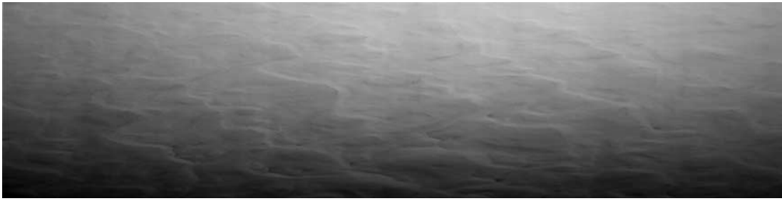
Figure 15a. A raw image from the Descent camera, acquired with a 5.1-ms exposure time over Kelso Dunes, California. The image was acquired at an altitude of 1200 m above the ground. This image is 1200 m wide by 1200 m high and the spatial resolution is 1.2 m/pixel horizontal and 4.8 m/pixel vertical. The image is brighter near the top due to the 5.1-ms shutter effect.
