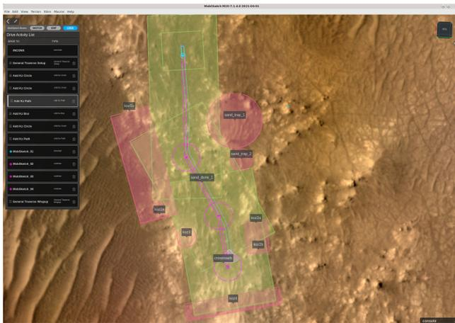
**Figure 10: MobSketch image showing the RP sketch of Sol 134 drive with directed and autonomous navigation segments. Also shown are the geometric Keep In Zones in green and Keep Out Zones in red which RPs create to keep AutoNav safe from non-geometric hazards that cannot be detected onboard.**
