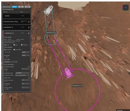
Figure 12: Example of a directed drive followed by an AutoNav drive. Here only the second leg is displaying the available options in the box on the left.
