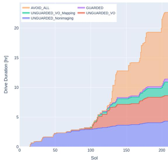
**Figure 20: Cumulative duration by drive mode.**
