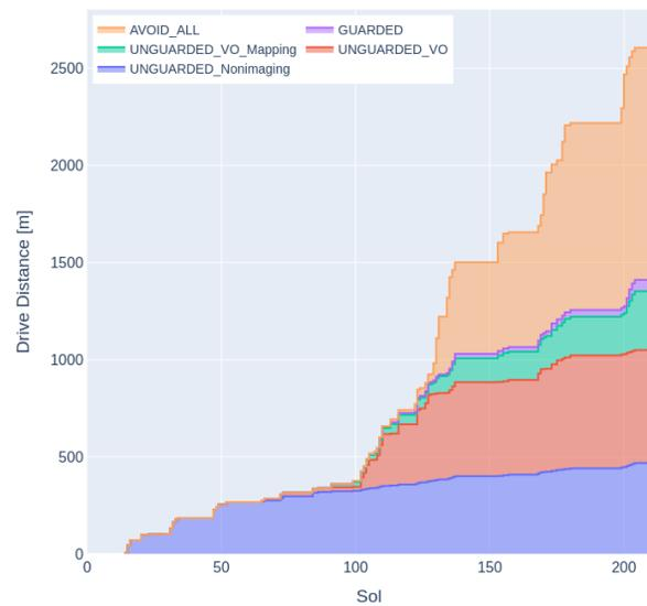
**Figure 19: Cumulative Odometry by drive mode for first 210 sols**
