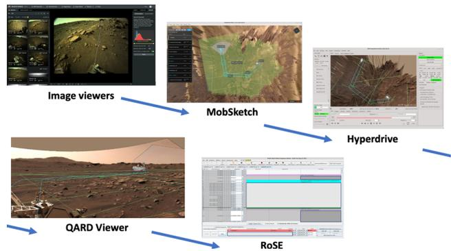
**Figure 8: Robotic Operations mobility tools and simplified high level workflow.**
