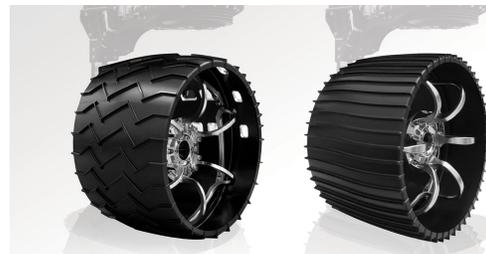
**Figure 5: Comparison of Curiosity (left) and Perseverance (right) wheels.**
