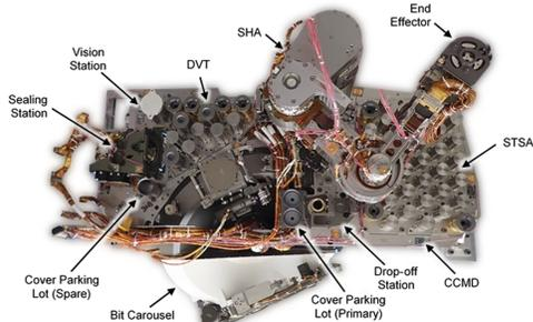
**Figure 6: Image of Adaptive Caching Assembly showing the stations with Sample Handling Arm deployed [4].**
