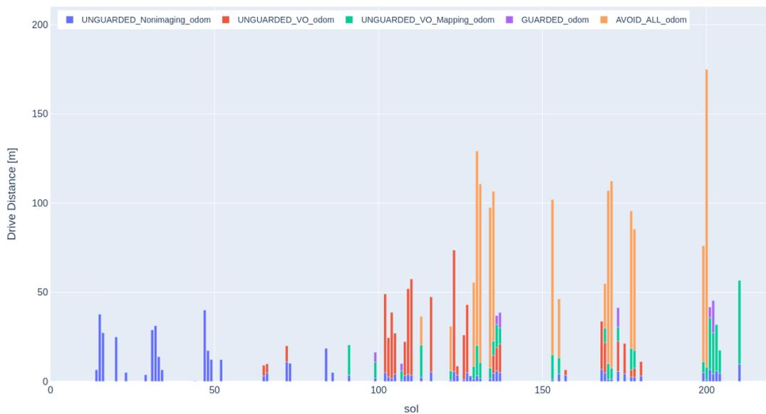
**Figure 21: Drive distance by drive mode for first 210 sols.**
