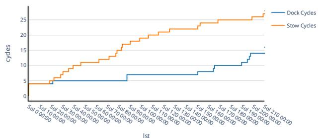
**Figure 27: Robotic arm stow and dock cycles.**
