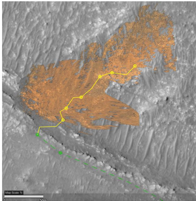
**Figure 29: Color images taken by Ingenuity overlaid over the planned strategic route of the Perseverance rover. The much higher resolution (images were taken 10m above ground) was very helpful to both the Science and RP teams for planning the Séítah toe dip.**
