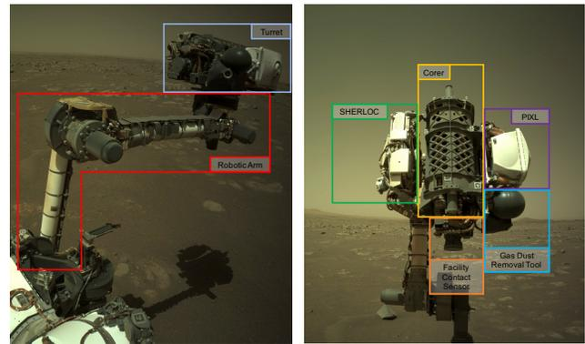
**Figure 3:** Components of the robotic arm and turret labeled in Navigation camera images.
