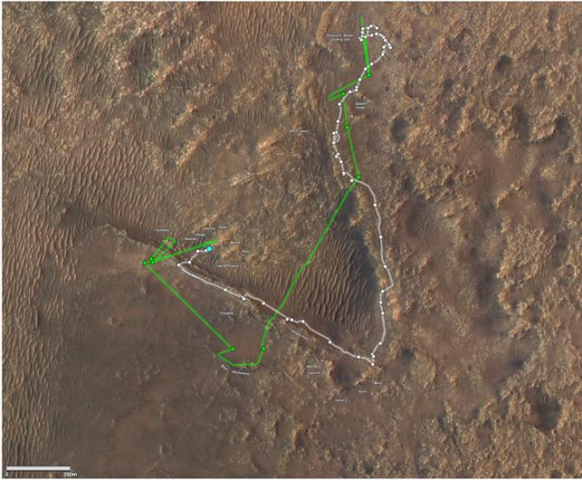
**Figure 2: Figure showing an Orbital map view of the Perseverance and Ingenuity paths as of Sol 210. Perseverance locations are shown in white and Ingenuity in green.**
