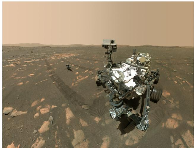
Figure 1: Perseverance and Ingenuity selfie taken by the rover on Sol 46 after deploying Ingenuity at Wright Brothers airfield and before the first flight.
